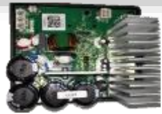
Variable Speed Drives
